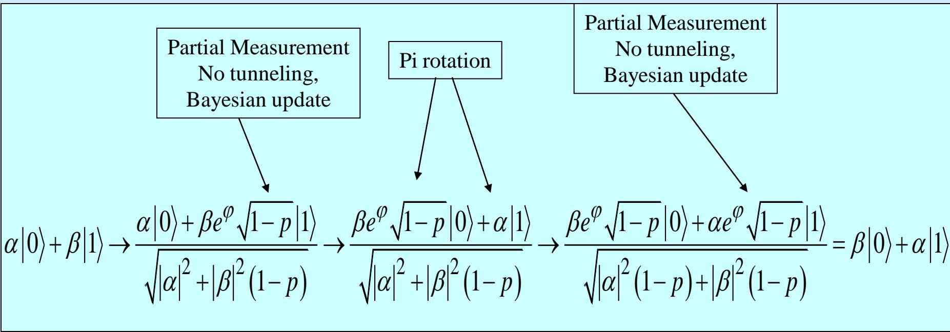
At each partial measurement there is a probability that the qubit will tunnel. Therefore, there is a probability that this procedure will destroy the qubit, otherwise you have performed a Pi rotation.
