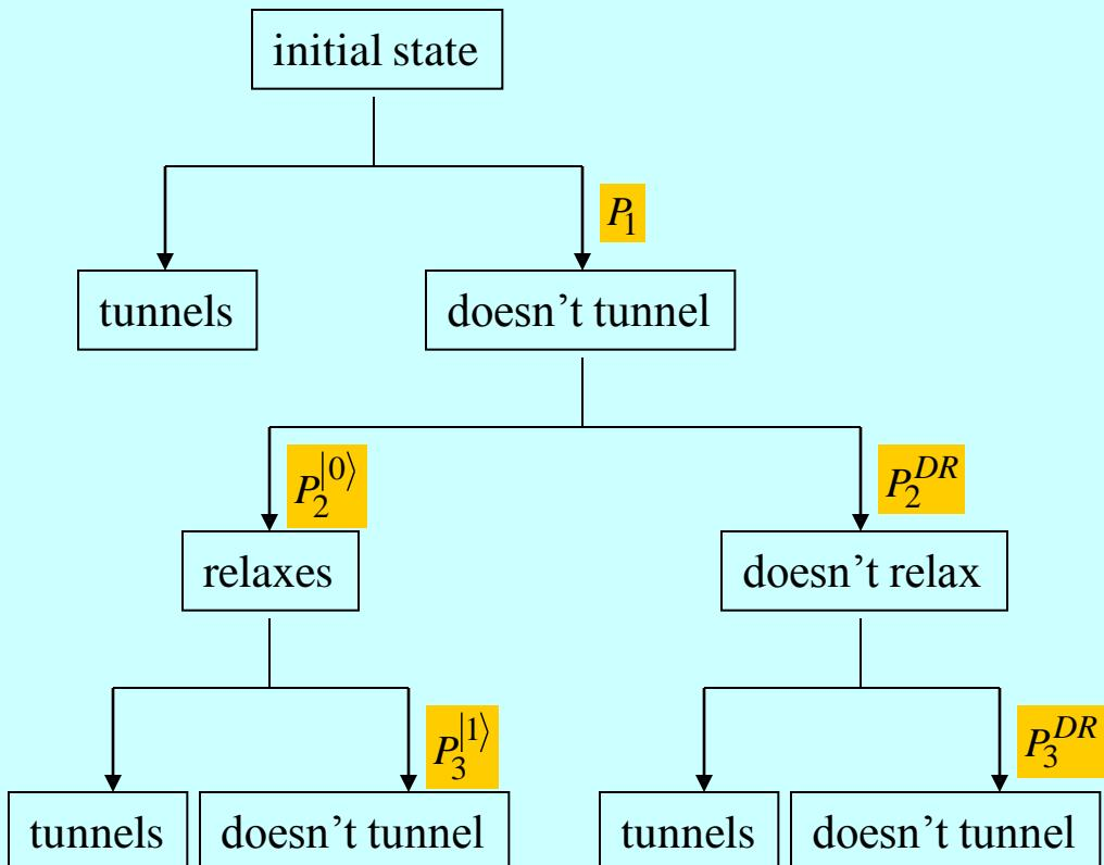
$$P_f^{[1]} = P_1 P_2^{[0]} P_3^{[1]} = |\beta|^2 (1-p)^2 \left(1 - e^{-t/T_1}\right) e^{-t/T_1}$$
