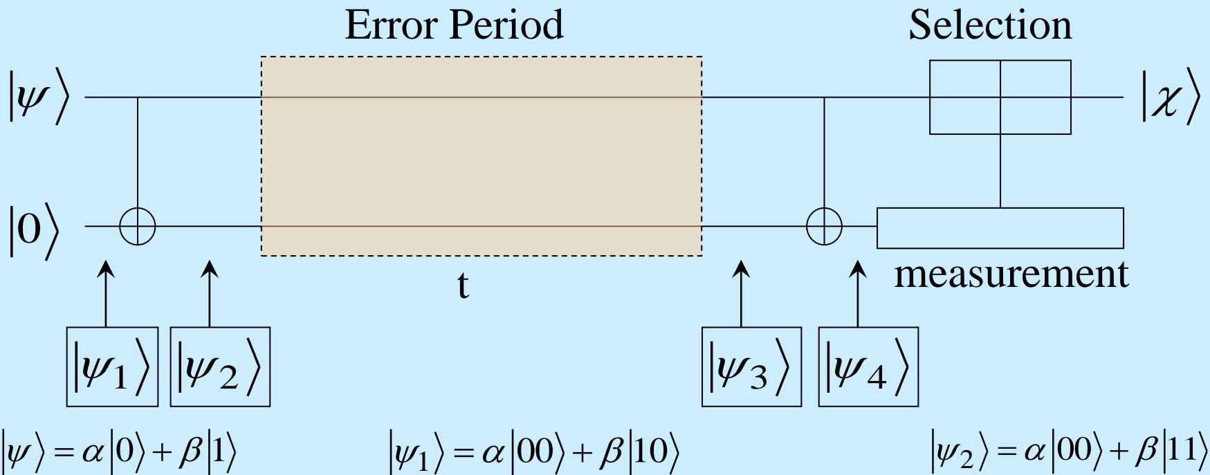
$$|\psi_3\rangle = \begin{cases} \frac{\alpha|00\rangle + \beta(1-p)|11\rangle}{\sqrt{|\alpha|^2 + |\beta|^2(1-p)^2}}, & \text{with prob. } P_{nor} = |\alpha|^2 + |\beta|^2(1-p)^2 \\ |10\rangle, & \text{with probability } P_{10} = |\beta|^2(1-p)p \\ |01\rangle, & \text{with probability } P_{01} = |\beta|^2 p(1-p) \\ |00\rangle, & \text{with probability } P_{00} = |\beta|^2 p^2 \end{cases}$$
